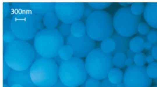
SEM image of polystyrene particle sample confirms the presence of three populations of 220nm, 400nm and 780nm diameter particles.
